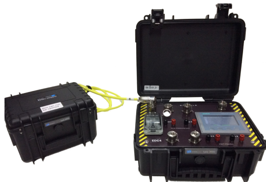
Control unit and 24V transformer/opt accumulator
